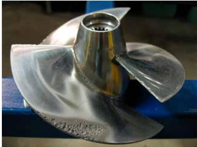
FIGURE 4 - Tip vortex and blade back cavitation (left), and cavitation damage (right)
