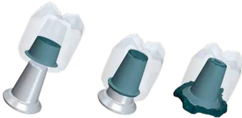
**FIGURE 5:** 3-D images generated in STAR-CCM+® showing the details of cement flow during crown seating on the CA
