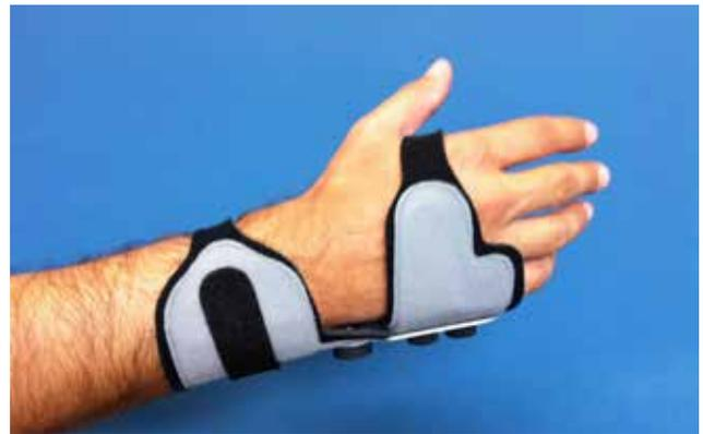
amplitude reduction with the final damper design was about eight to nine times higher than with the initial design. With the initial damper design, the reduction in amplitude seemed to increase with decreasing frequency contrary to the target characteristics. With the final damper design, the maximum amplitude reduction was around 2 Hz, and reducing with decreasing frequency below this level.
