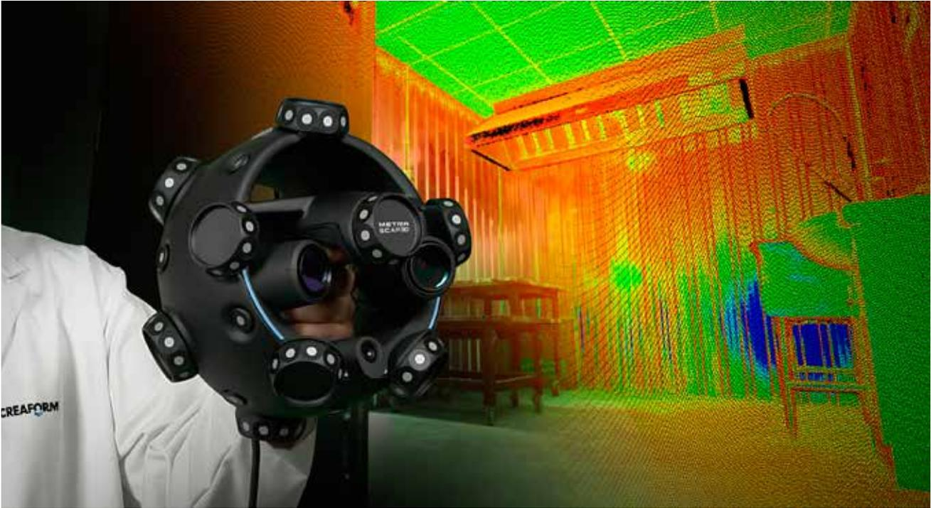
**FIGURE 2:** Room scan using Creafom's handheld MetraSCAN
