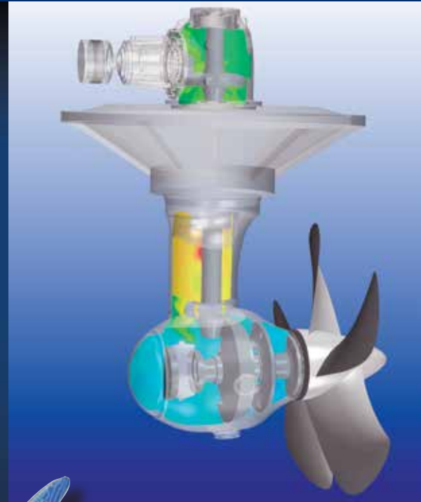
Above: Temperature field of the oil in an azimuth thruster. Image courtesy of VICURA.
