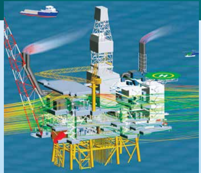
Above: CFD is routinely used to predict, quantify and mitigate some of the risks associated with floating and fixed offshore structures.
